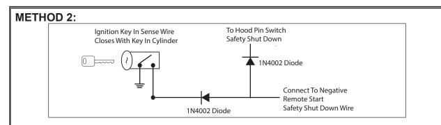
To connect to the key in sensor circuit as shown for method 2:
