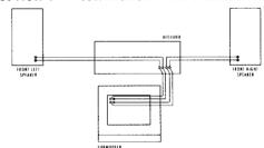
Connect speaker wires from the Receiver's Front Left and Right Speaker Outputs to the Subwoofer's SPEAKER-IN terminals. Connect Left channel to Left, and Right channel to Right. The connections to the Subwoofer are in parallel with the wires from your Receiver to your Front Speakers.
